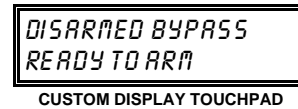
TYPICAL DISPLAYS AFTER ALL BYPASSED ZONES HAVE BEEN DISPLAYED (PRIOR TO ARMING)
